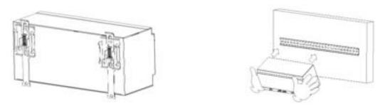
Step 2: Place the upper hooks of DIN Rail Brackets onto the upper edge of DIN Rail, push and hold down the spring-loaded bars on the DIN Rail Brackets, then push the bottom of UPS forward against the DIN Rail, and finally release the spring-loaded bars.
