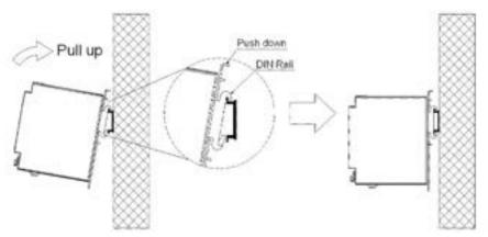
Step 3: Slightly pull the bottom of the UPS outward to ensure that the spring loaded hooks are securely engaged onto the lower edge of the DIN Rail.
