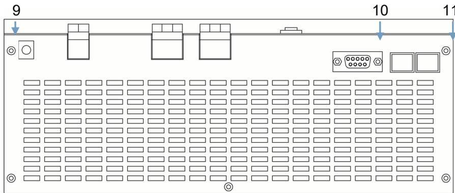
**9. AUX DC OUTPUT:** Output terminal provides DC power source to the relay card (Optional Dry contact relay box).
