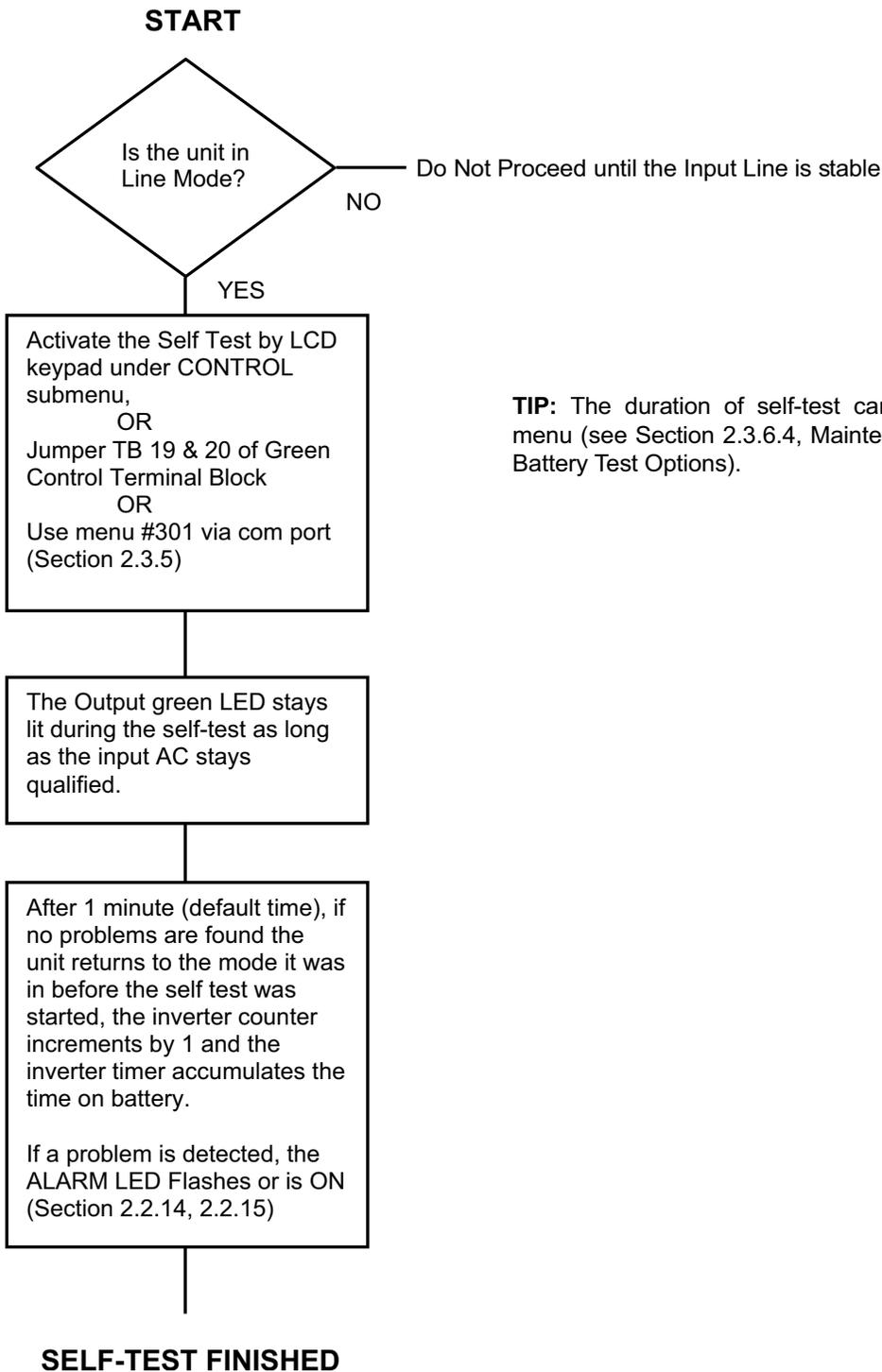
**TIP:** The duration of self-test can be adjusted via menu (see Section 2.3.6.4, Maintenance Menu # 30, Battery Test Options).
