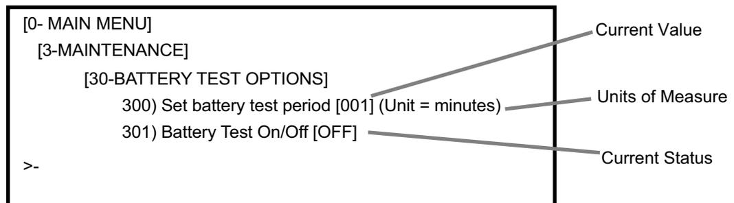
To calculate the Test Period: Test Period = Current Value X Units
