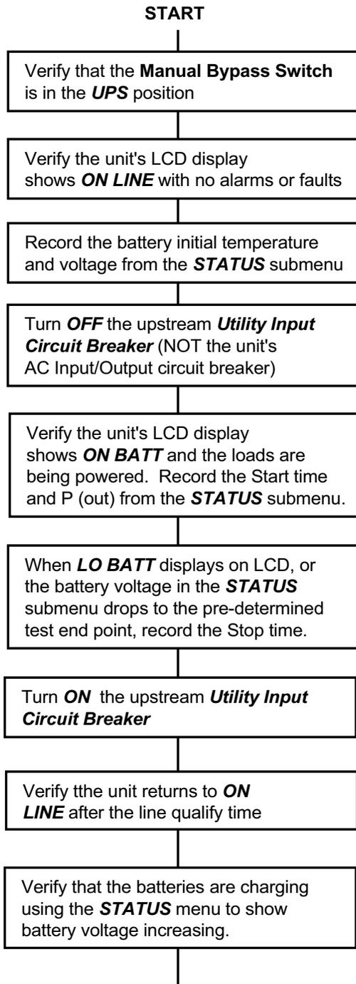
**TIP:** The event log can be used via the com port to record the battery initial voltage on float, the battery initial temperature, time the unit went On Batt and when the Lo Batt alarm occurred.
