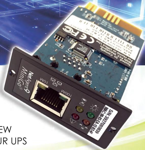
NetAgent Mini integrates multi-network communication protocols to enable a comprehensive, easy-to understand and secure remote monitoring and management for UPS and other equipment via the internet.
