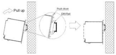
Step 3: Slightly pull the bottom of the UPS outward to ensure that the spring loaded hooks are securely engaged onto the lower edge of the DIN Rail.
